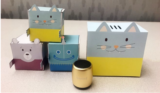
Figure 2: On the left, static versions of voice agents we called miniBear, miniCat and miniBot. On the right, the portable tangible voice agent with closed top and Bluetooth speaker on the front.
